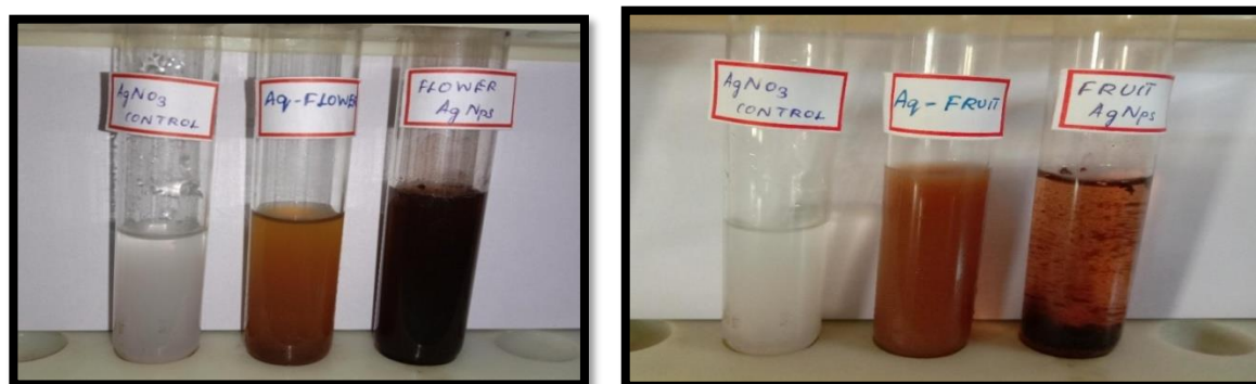
Figure 1: Biosynthesis of silver nanoparticles. a) Formation of V. inermis flower SNPs b) Formation of V. inermis fruit SNPs
